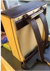
smaller improvements the new CAD-data was sent to a special metal worker who lasered the mechanical parts from 2mm thick brass and gave it to our group for a good price and nice quality.
